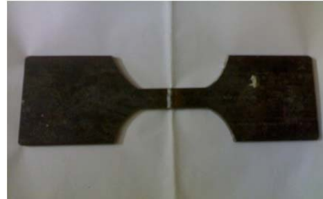
Fig. 5: Tensile test specimen as per ASTM standard
